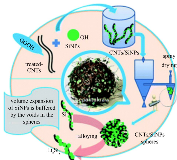
图8 喷雾干燥法制备一种硅碳纳米管(CSs)复合材料原理 Fig.8 A Si-CNTs (CSs) composite material was prepared by spray drying
